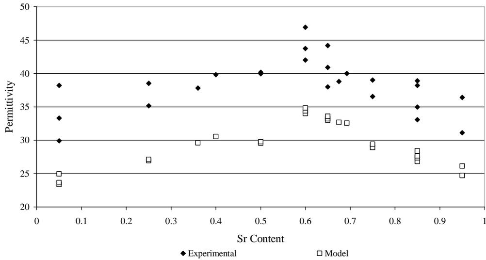
Fig. 7. Comparison of measured permittivity and calculation using ion compression model for materials with “ $t$ ” > 0.995.
