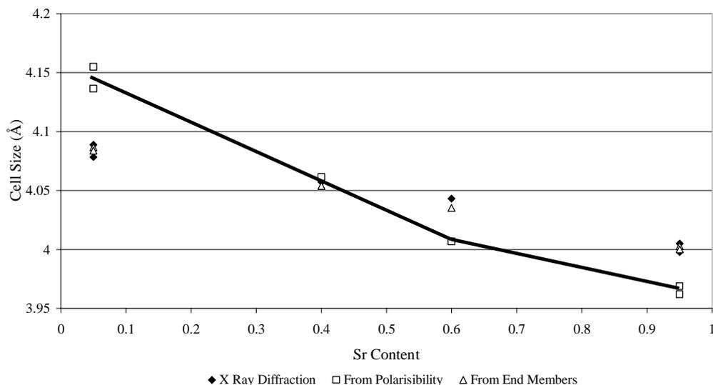
Fig. 5. Cell size calculated by various routes.
