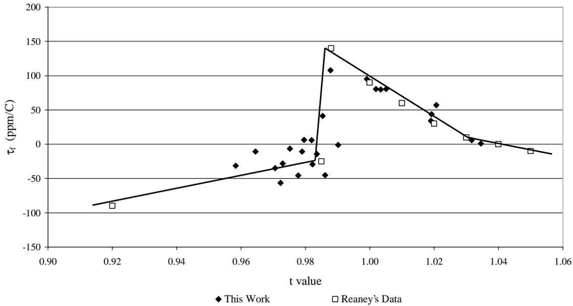
Fig. 1. Temperature coefficient of resonant frequency and “*t*” factor.
