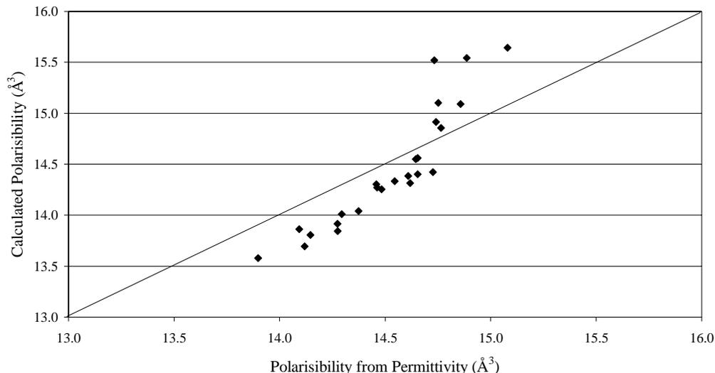
Fig. 3. Comparison of polarisibility calculated from permittivity and from ion additivity rule.
